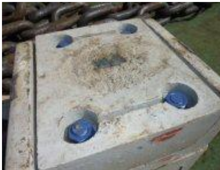
The clump weights were designed and manufactured by Monobuoy using a Vietnamese casting and forging company. Over 800 tonnes of clump weights were needed for the mooring system.
