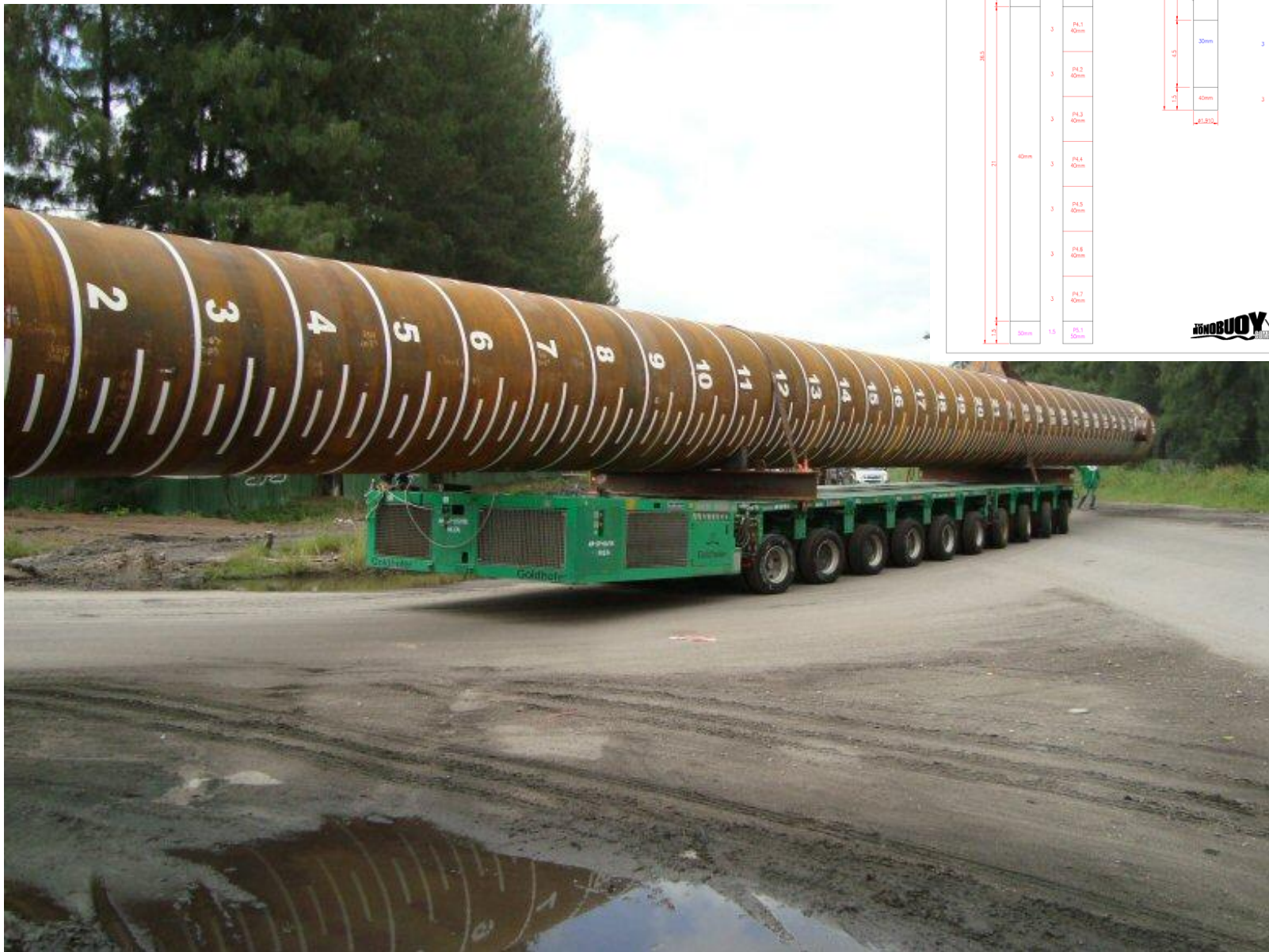
9 anchor piles were designed and manufactured by Monobuoy in 3 months in a Malaysian fabrication yard.
